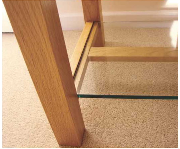
▲ Pic.4 The lower rails are rebated to receive the 8mm plate glass shelf
